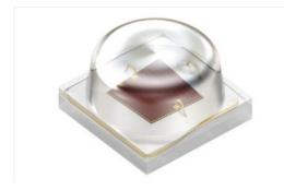
From the OSLON Square family comes the OSLON Square Batwing. This product solves a problem encountered in greenhouses all over the world. Current LED fixtures using lambertian primary lens and a glass cover are at risk of creating hotspots of high concentrations of light directly underneath the fixture. The primary optics on the OSLON Square Batwing increase light uniformity, enabling design simplification, fixture count reducation and increased efficiency.
